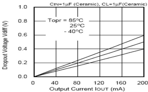
4、Dropout Voltage vs. Output Current
