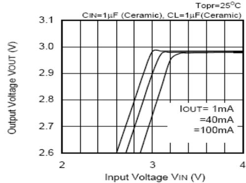
3、Dropout Voltage vs. Output Current
