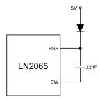
This diode is also recommended for high duty cycle operation and high output voltage applications.
