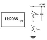
Select the proper ratio of the two feedback resistors  $R_{FB1}$  and  $R_{FB2}$  based on the output voltage. Adding a capacitor in parallel with  $R_{FB1}$  helps the system stability. Typically, use  $R_{FB2} \approx 10 k\Omega$  and determine RFB1 from the following equation:
