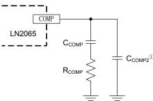
NOTE ①: C<sub>COMP2</sub> is needed only for high ESR output capacitor
