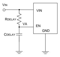
For example, setting  $V_{\text{IN}}$ =24V,  $R_{\text{DELAY}}$ =100K $\Omega$ ,  $C_{\text{DELAY}}$ =0.1uF. The start-up delay time can be calculated as below:
