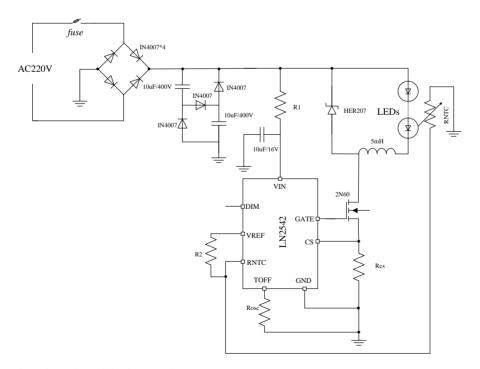
Note: 1. R1 is based on the value of the Input voltage.
