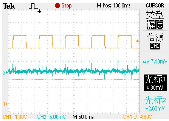
13. Input voltage transient response (IL=10mA)
