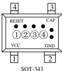
① ② represent the Output type and Voltage threshold.
