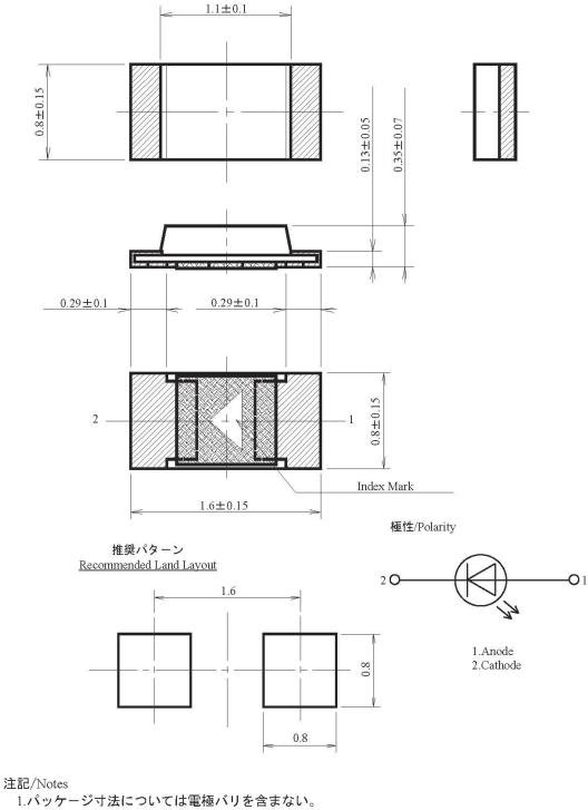
Measurement of the package doesn't include electrode projection.
