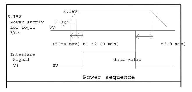
\* Set 0 Volt < Vi(t) <  $V_{DD}(t)$  Here Vi(t),  $V_{DD}(t)$  indicate the transitive state of Vi,  $V_{DD}$  when power supply is turned
