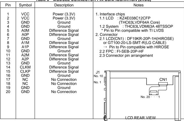
The B/L inverter interface connector is a model 52271-1090 10P, manufactured by Molex or equivalent FPC connector. The pin configuration of the J1 connector is shown in the table below.
