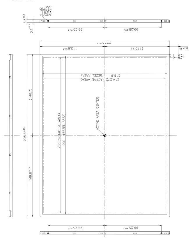
Notes 1. Unspecified dimensional tolerance are  $\pm 0.5 \text{mm}$
