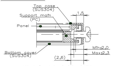
\* Mounting Screw depth: 2.0[mm] Min. 2.3[mm] Max.
