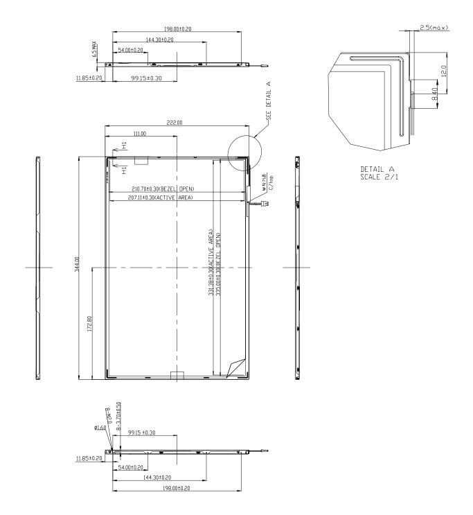
Note. unspecified dimensional tolerance are +/-0.5mm
