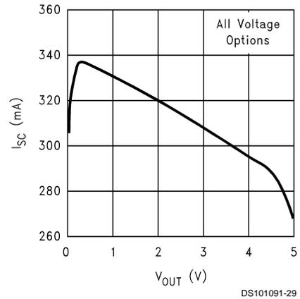
**Typical Performance Characteristics** Unless otherwise specified:  $T_A = 25^\circ\text{C}$ ,  $C_{OUT} = 4.7 \mu\text{F}$ ,  $C_{IN} = 1 \mu\text{F}$ , ON/OFF pin tied to  $V_{IN}$ ,  $V_{IN} = V_{O(NOM)} + 1\text{V}$ ,  $V_{OUT(NOM)} = 1.8\text{V}$ . (Continued)
