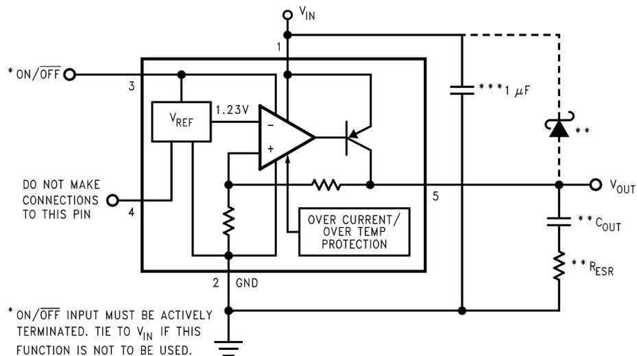
\* ON/OFF INPUT MUST BE ACTIVELY TERMINATED. TIE TO  $V_{IN}$  IF THIS FUNCTION IS NOT TO BE USED.
