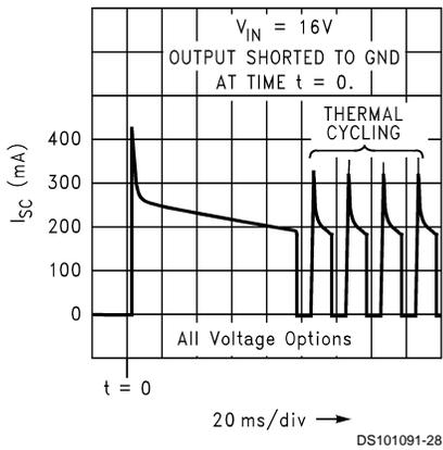
**Instantaneous Short Circuit Current vs Output Voltage**
