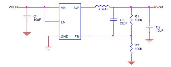
Adjustable Voltage Application Circuit
