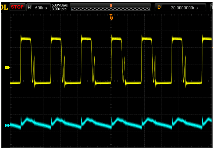
V_{IN}=5V, V_{OUT}=12V, I_{OUT}=100mA, CH_1=V_{SW}, CH_2=\Delta V_{OUT}
