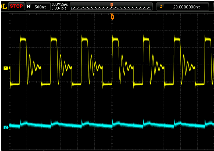
V_{IN}=5V, V_{OUT}=12V, I_{OUT}=50mA, CH_1=V_{SW}, CH_2=\Delta V_{OUT}
