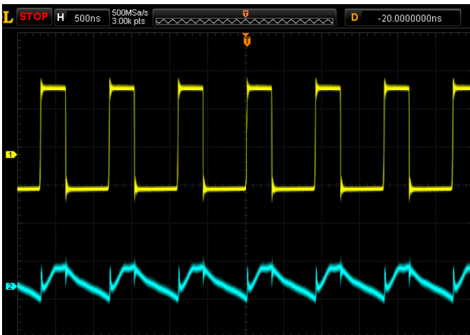
V_{IN}=5V, V_{OUT}=12V, I_{OUT}=300mA, CH_1=V_{SW}, CH_2=\Delta V_{OUT}
