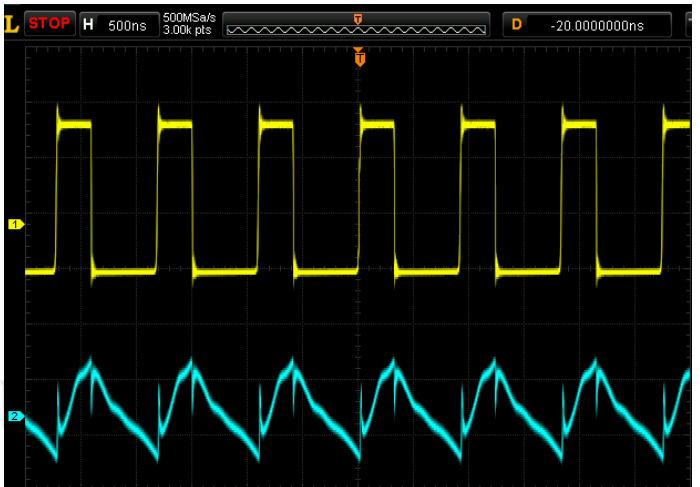
V_{IN}=5V, V_{OUT}=12V, I_{OUT}=600mA, CH_1=V_{SW}, CH_2=\Delta V_{OUT}
