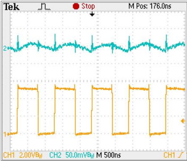
V_{OUT}=5V, V_{IN}=3V, I_{OUT}=500mA, CH_1=V_{SW}, CH_2=\Delta V_{OUT}
