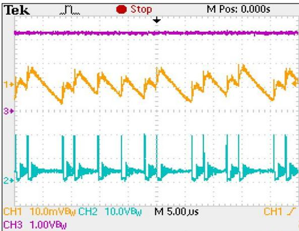
$V_{IN}=16V, V_{OUT}=3.3V, I_{OUT}=50mA$
