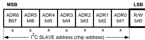
Figure 50. Address and Read/Write Bit
