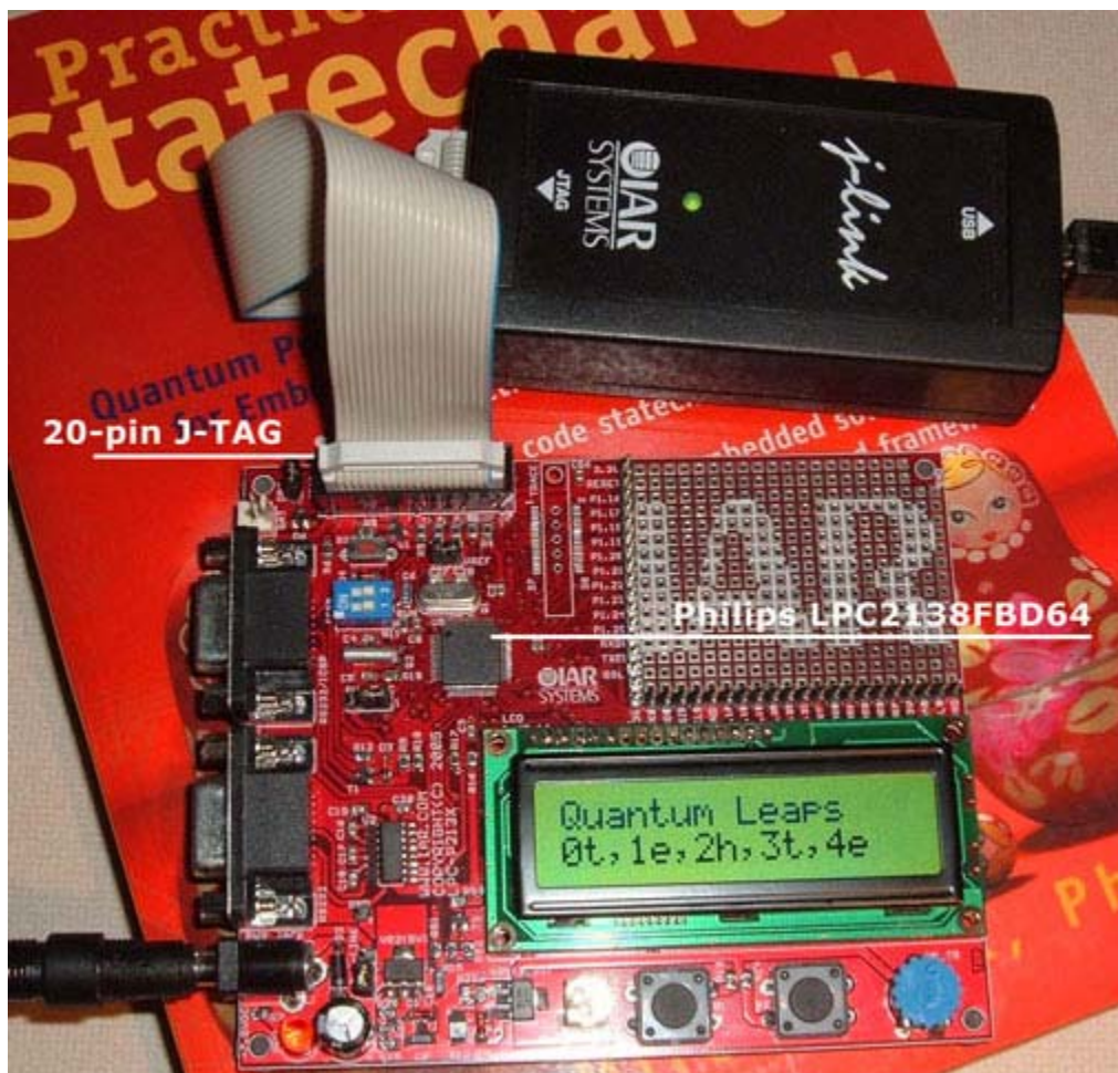
Figure 1 IAR KickStart Kit including the LPC-P213x Evaluation Board and the J-Link J-TAG pod from Segger, GmbH.
