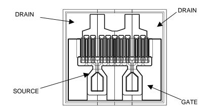
DIE SIZE: 16.5 x 16.1 mils (420 x 410 μm) DIE THICKNESS: 3.0 mils (75 µm typ.)
