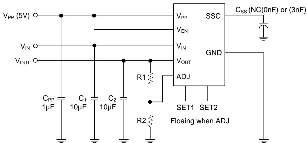
$$V_{OUT} = \frac{0.8(R_1+R_2)}{R_2} \text{ Volts}$$
