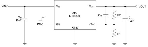
Cff option notes: the capacitance of feed-forward capacitor with range of 10pF to 1uF allows to achieve better PSRR performance when required by the application
