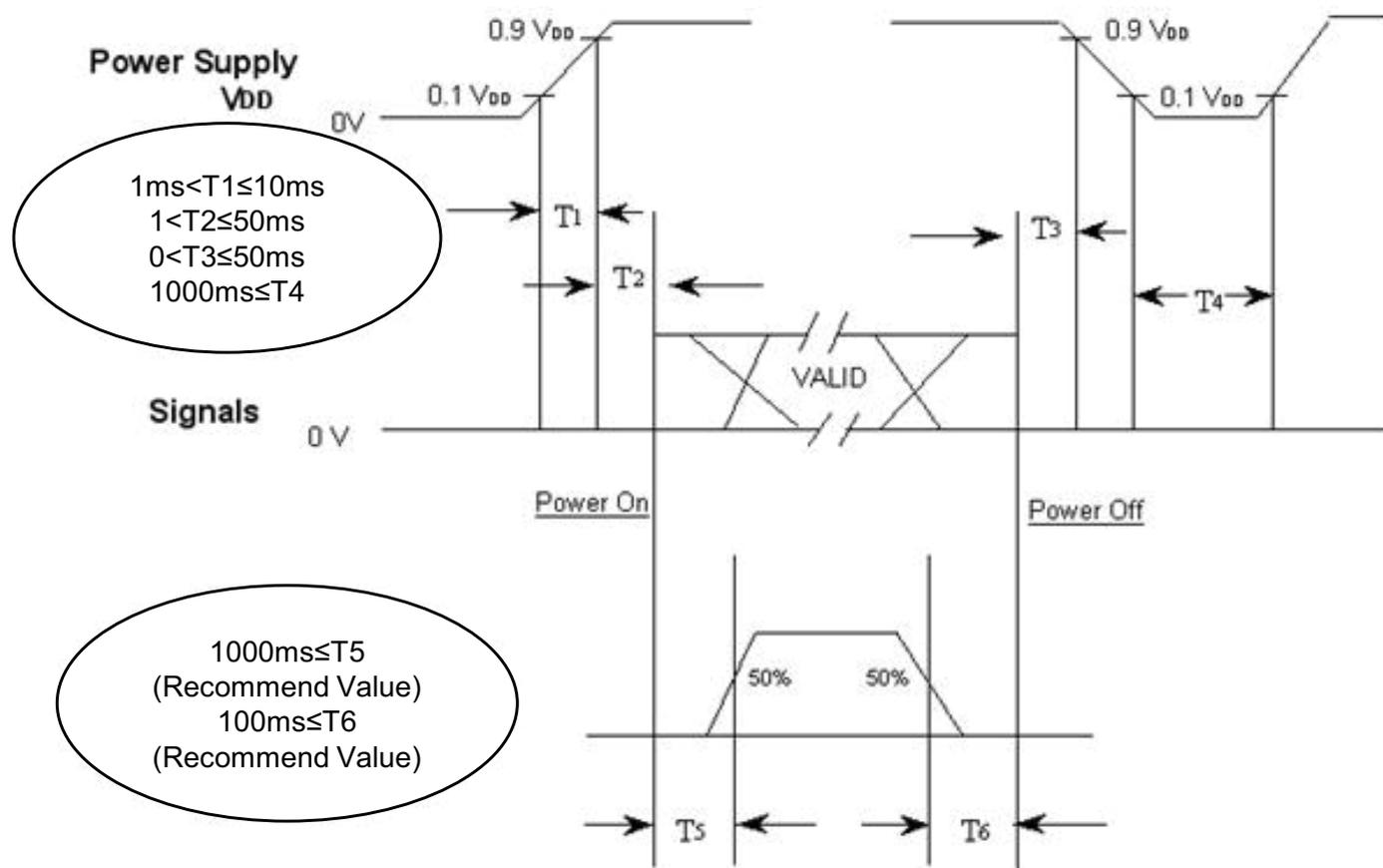
T1 :  $V_{DD}$  rising time from 10% to 90%
