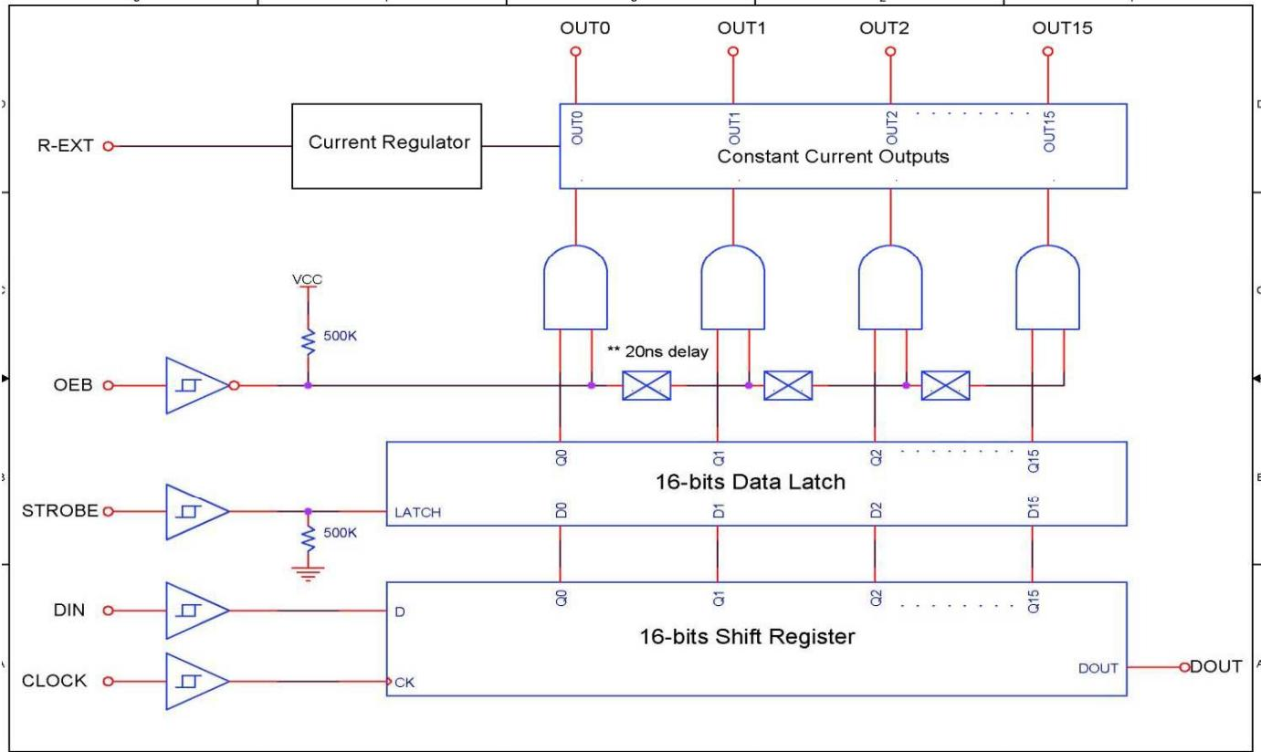
This is designed for high speed switching between outputs and is intended to have the effect of reducing switching noise when all outputs are ON or OFF at the same time.
