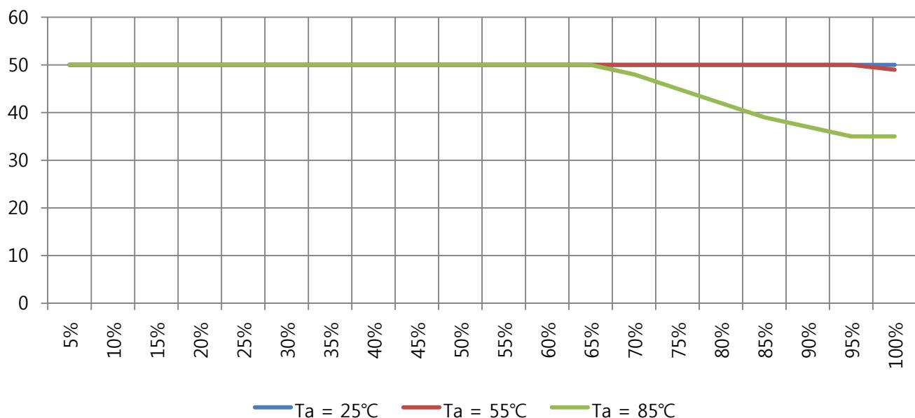
Due to above curve, when SSOP24 type package in operating  $I_{out(max)} = 50\text{mA}$  LSD9016-X24T is adviced to choice duty cycle, around 65%.
