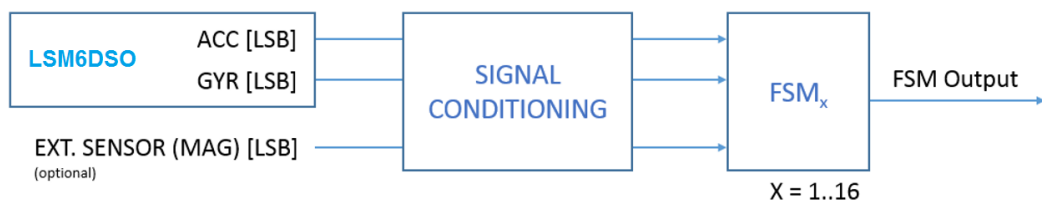
Figure 2. State machine in the LSM6DSO
