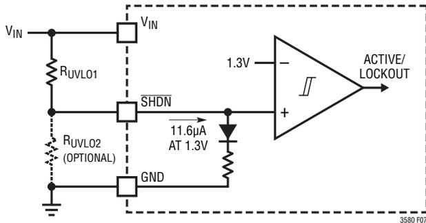
Figure 7. Configurable UVLO
