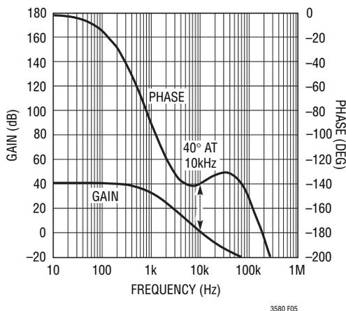
**Figure 5. Bode Plot for Example Boost Converter**
