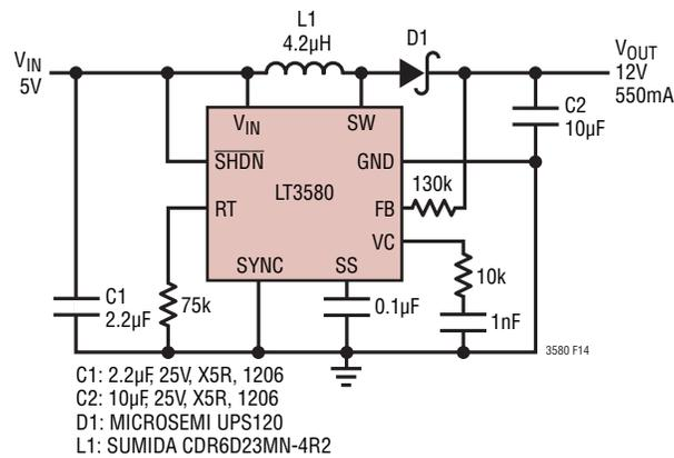
Figure 14. 1.2MHz, 5V to 12V Boost Converter
