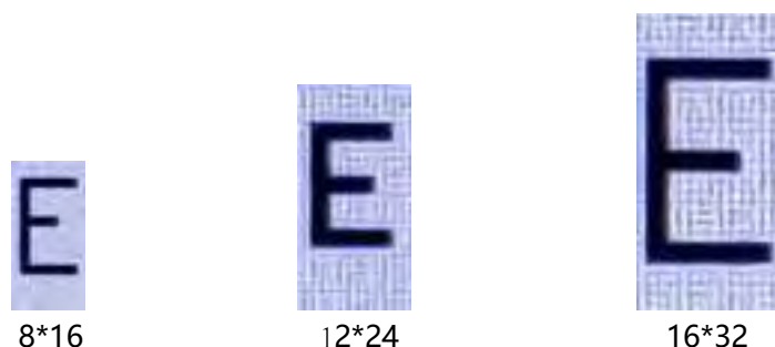
Figure 8-1B: Internal ASCII Font for 8*16, 12*24 and 16*32
