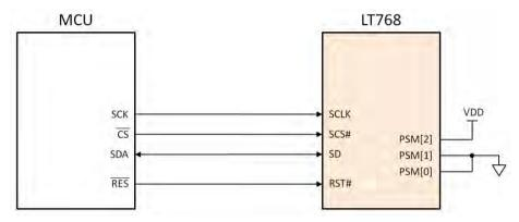
Figure 2-5: 3-Wire SPI Interface
