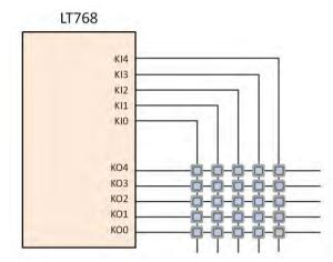
Figure 11-1: Application Circuit of Keypad-scan
