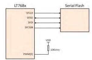
Figure 10-1: Enable the "Power-On Display" Function
