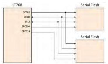
Figure 10-4: Application Circuit of Serial Flash/ROM
