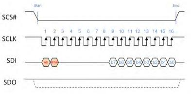
Figure 2-8: 4-Wire SPI Interface Write Timing
