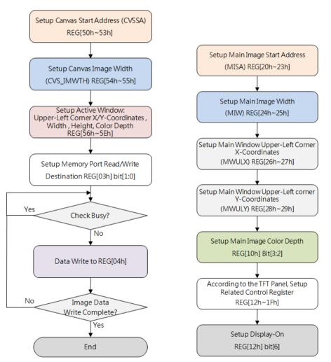
Figure 5-3: Write Image Data to Display Image Buffer
