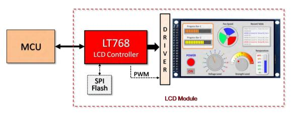
Figure A-3: LT768x Designed on TFT-LCD Module
