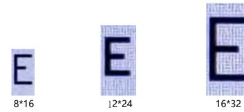
Figure 8-1B: Internal ASCII Font for 8\*16, 12\*24 and 16\*32
