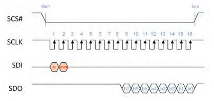
Figure 2-9: 4-Wire SPI Interface Read Timing
