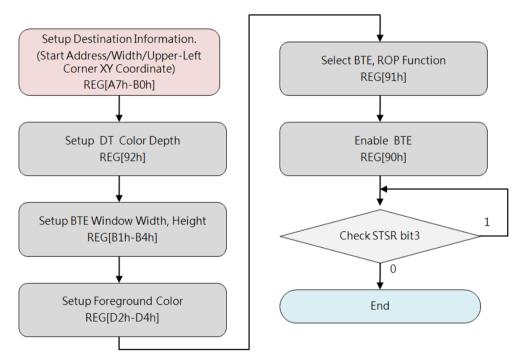
Figure 7-39: Flow Chart of Solid Fill
