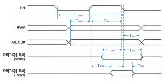
Figure 2-4: 6800 Parallel Mode Interface Timing
