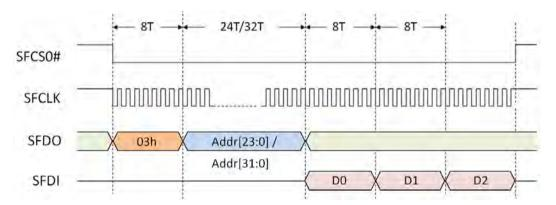
Figure 10-6: Normal Read Command of SPI Flash
