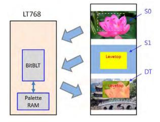
Figure 7-25: Example of Pixel Mode - 8bpp
