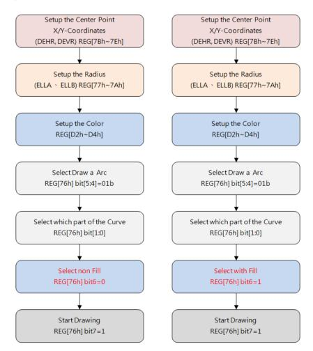
Figure 6-4: Flowchart of Drawing Curve and one-fourth Ellipse
