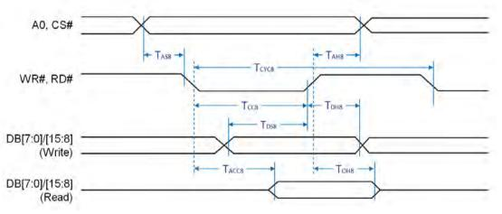
Figure 2-2: 8080 Parallel Mode Interface Timing
