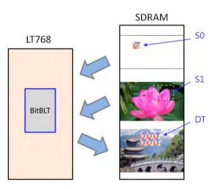
Figure 7-14: Example of Pattern Fill with ROP
