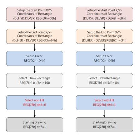
Figure 6-6: Flowchart of Drawing a Rectangle
