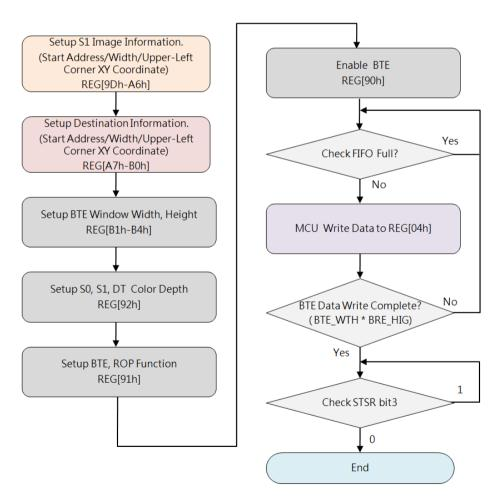
Figure 7-31: Flow Chart of MCU Write with Opacity
