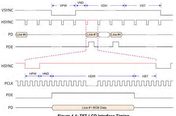
Figure 4-1: TFT-LCD Interface Timing
