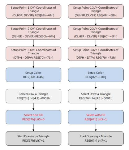
Figure 6-9: Flowchart of Drawing a Triangle
