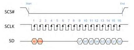
Figure 2-6: 3-Wire SPI Interface Timing
