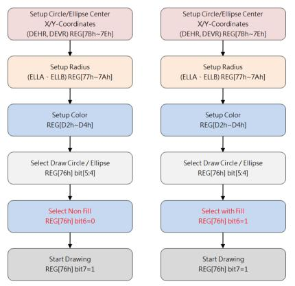
Figure 6-2: Flowchart of Drawing Circle and Ellipse
