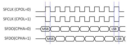
Figure 10-2: Master SPI Data Transfer
