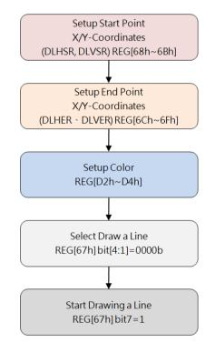
Figure 6-7: Flowchart of Drawing a Line
