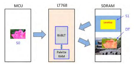
Figure 7-30: Example of MCU Write with Opacity
