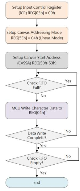
Figure 8-2: Flow Chart of CGRAM Initialization from MCU
