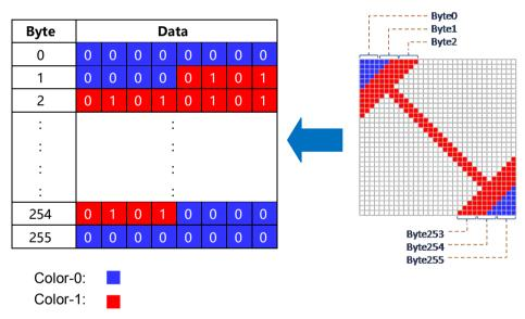
Figure 8-11: Graphic Cursor Data Format and Example
