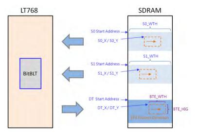
Figure 7-3: BTE Memory Access Method
