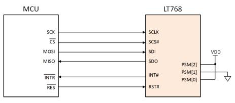
Figure 2-7: 4-Wire SPI Interface
