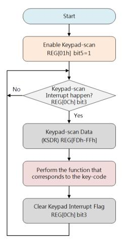
Figure 11-2: Flowchart to check Key-pad Interrupt (S/W Polling Mode)
