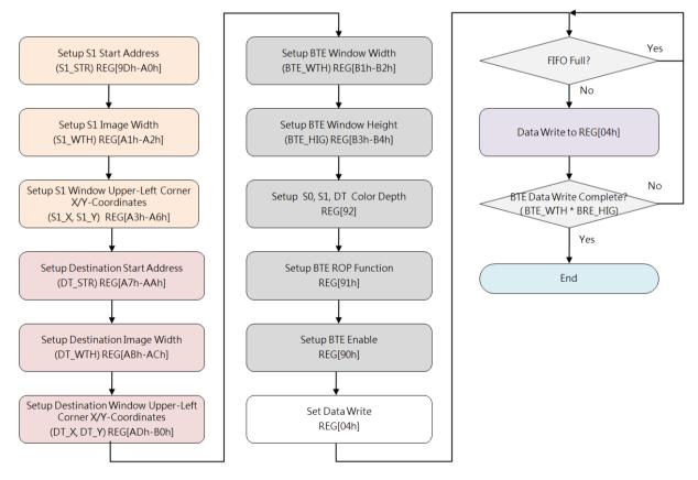
Figure 7-5: Flow Chart of MCU Wtite with ROP
