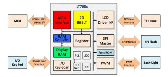
Figure A-1: Internal Block Diagram
