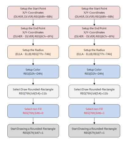
Figure 6-11: Flowchart of Drawing a Rounded-Rectangle
