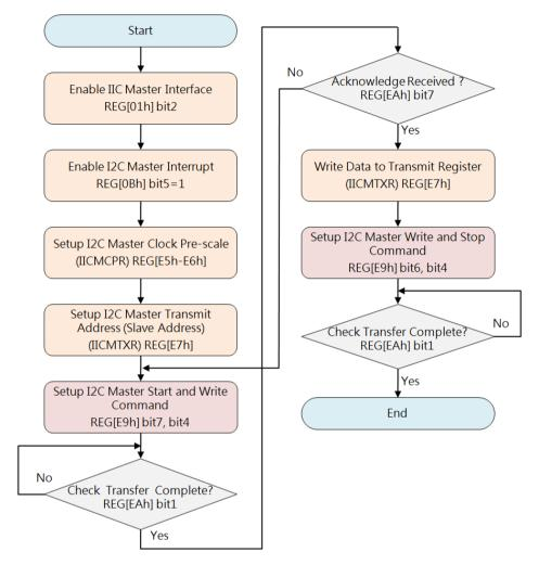
Figure 10-16: Write Data to Slave
