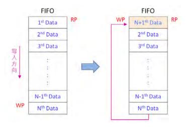
Figure 10-3: FIFO Overrun Example
