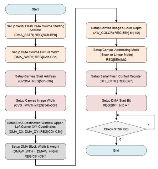
Figure 10-12: DMA Data Transfer Flowchart (Polling Mode)
