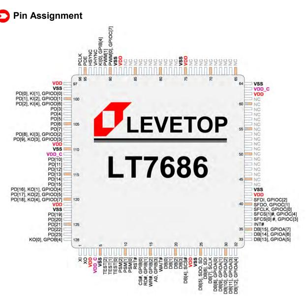
Figure A-4: LT7681/LT7683+/LT7686 Pin Assignment (LQFP-128Pin)
