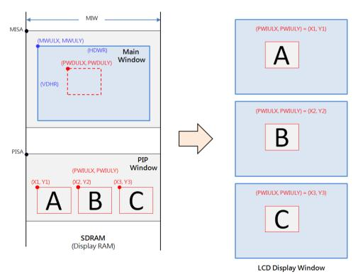
Figure 5-7: Select Different PIP image on the Screen
