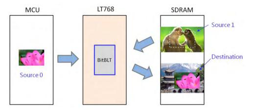
Figure 7-4: Example of MCU Write with ROP
