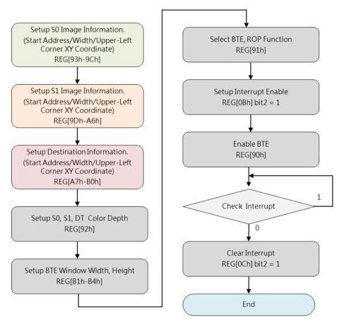
Figure 7-8: Flow Chart 2 of Memory Copy with ROP
