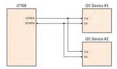
Figure 10-14: Application Circuit of LT768x I2C Master
