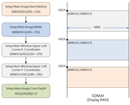
Figure 5-4: Setup and Select Main Window Image
