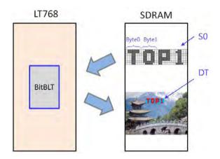
Figure 7-32: Example of Memory Copy with Color Expansion
