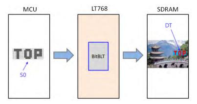
Figure 7-18: Example of MCU Write with Color Expansion
