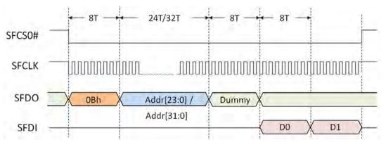
Figure 10-7: SPI Fast Read Command of SPI Flash
