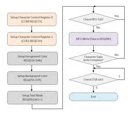
Figure 8-1: Flow Chart of CGROM Basic Programming
