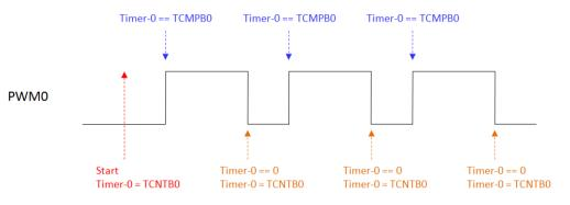
Figure 9-1: PWM0 Output Wave Form
