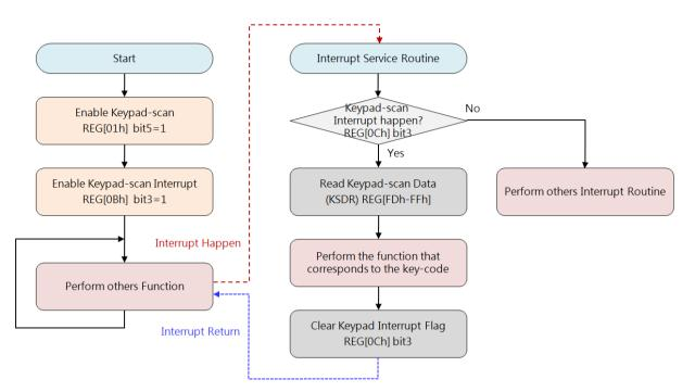
Figure 11-3: Flowchart to check Key-pad Interrupt (H/W Interrupt Mode)
