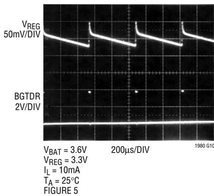
**Regulator Output Transient Response—Wall Adapter Removal**
