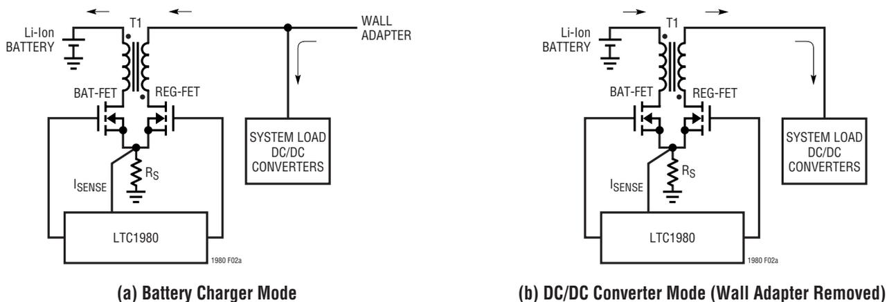
Figure 2. LTC1980 Bidirectional Power Conversion
