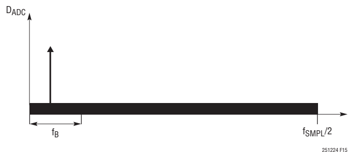
Figure 15. Frequency Spectrum of SAR ADC Core Output
