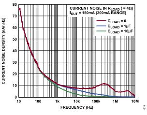
Figure 22. Current Noise Density vs. Frequency, Grounded C<sub>LOAD</sub> = 0 µF, 1 µF, and 10 µF
