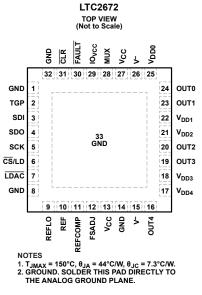
Figure 5. LFCSP Pin Configuration
