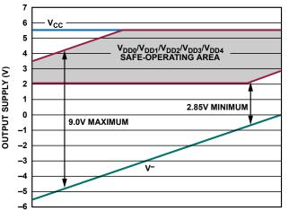
Figure 33. Output Supply Safe Operating Area
