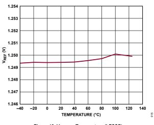
Figure 18. V<sub>REF</sub> vs. Temperature (LFCSP)
