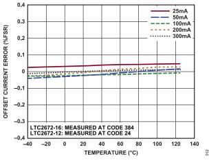
Figure 15. Offset Current Error vs. Temperature
