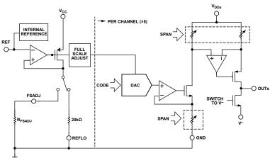
Figure 28. Single-Channel Simplified Diagram
