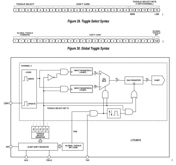
Figure 31. Conceptual Block Diagram, Toggle Functionality
