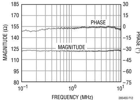
Figure 12. Termination Magnitude and Phase vs Frequency
