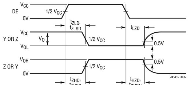
Figure 5. Driver Enable and Disable Timing Measurements
