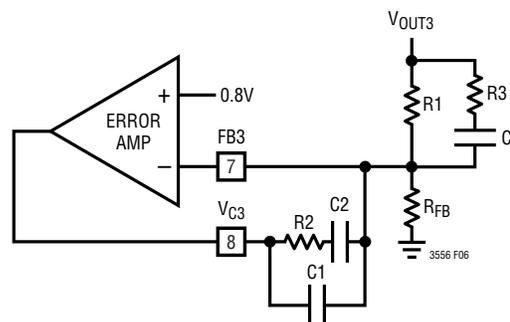
Figure 6. Error Amplifier with Type III Compensation
