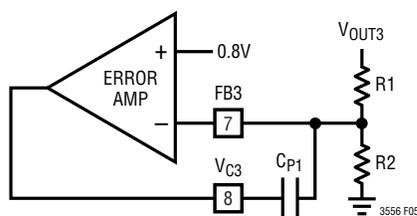
Figure 5. Error Amplifier with Type I Compensation
