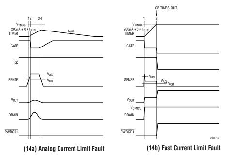
Figure 14. Current Limit Behavior (All Waveforms are Referenced to V<sub>EE</sub>)
