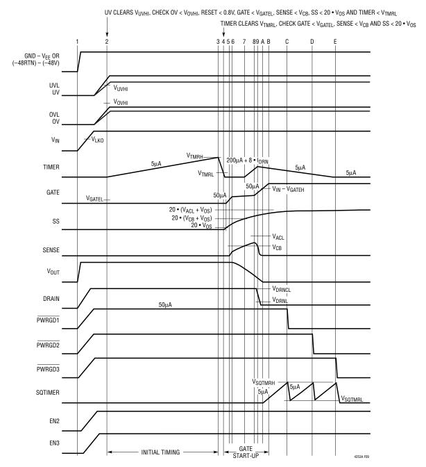
Figure 9. Power-Up Timing with a Short Pin (All Waveforms are Referenced to V<sub>EE</sub>)
