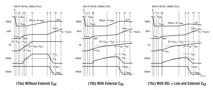
Figure 15. Soft-Start Timing (All Waveforms are Referenced to VEE)
