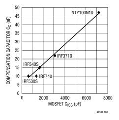
Figure 6. Recommended Compensation Capacitor C<sub>C</sub> vs MOSFET C<sub>ISS</sub>
