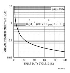
Figure 3. Circuit Breaker Response Time
