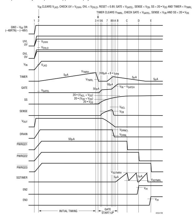
Figure 8. System Power-Up Timing (All Waveforms are Referenced to V<sub>FF</sub>)
