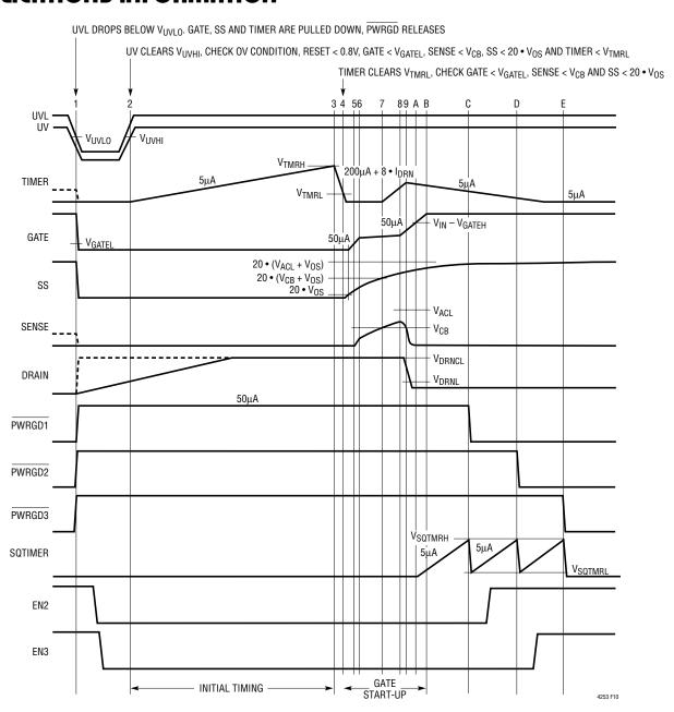
Figure 10. Undervoltage Timing (All Waveforms are Referenced to V<sub>EE</sub>)
