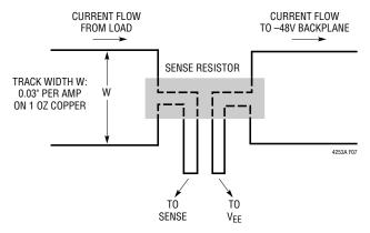
Figure 7. Making PCB Connections to the Sense Resistor
