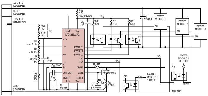
Figure 1. -48V/2.5A Application with Operating Range from 43V to 82V
