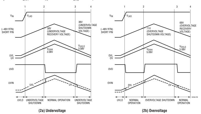
Figure 2. Undervoltage/Overvoltage Recovery and Shutdown (All Waveforms are Referenced to V<sub>FF</sub>)
