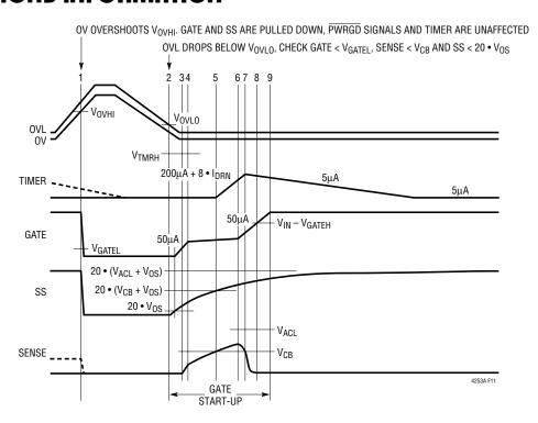
Figure 11. Overvoltage Timing (All Waveforms are Referenced to V<sub>FF</sub>)
