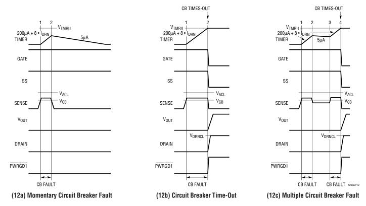
Figure 12. Circuit Breaker Timing Behavior (All Waveforms are Referenced to V<sub>FF</sub>)
