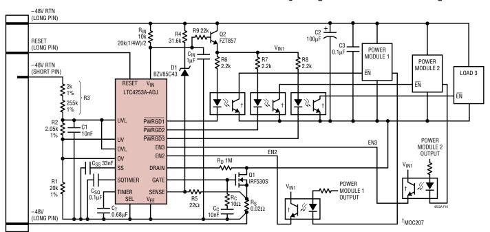
Figure 16. Power Limit Circuit Breaker Application
