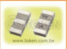
The dimensions of LTCA/CV10.7M ceramic chip filter is small as  $7.0\pm0.3 \times 3.0\pm0.3$  mm with low profile  $1.5\pm0.2$  mm. Insertion Loss max(dB) is from 3.0 db ~ 10 db, Spurious Attenuation (9~12 MHz) min(dB) 30 db ~ 35 db with Input/Output Impedance:  $330\Omega$ . Various bandwidths are available. Select a suitable type in accordance with the desired selectivity.
