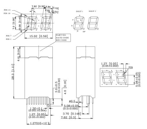
NOTES: 1. All dimensions are in millimeters. Tolerances are  $\pm$  0.25 mm unless otherwise note. 2. Pin tip's shift tolerance is  $\pm$  0.4 mm.
