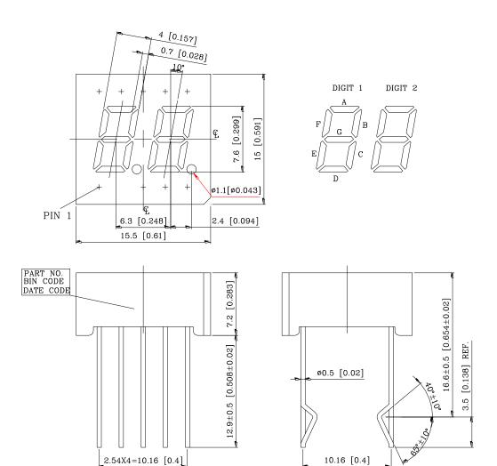
NOTES: All dimensions are in millimeters. Tolerance are  $\pm$  0.25 mm (0.01") unless otherwise noted.
