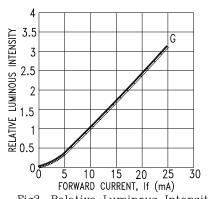
$\begin{array}{cccc} Fig3. & Relative & Luminous & Intensity \\ & vs. & DC & Forward & Current \end{array}$
