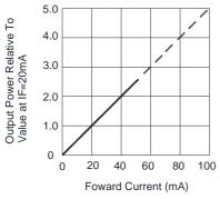
FIG.5 RELATIVE RADIANT INTENSITY VS. FORWARD CURRENT
