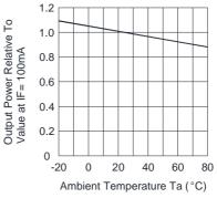
FIG.4 RELATIVE RADIANT INTENSITY VS. AMBIENT TEMPERATURE
