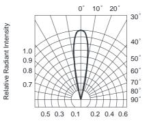
FIG.6 RADIATION DIAGRAM
