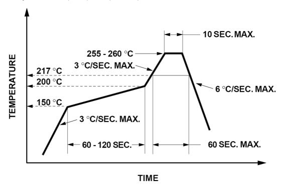
You can use this example as a generic target to set up your reflow process.
