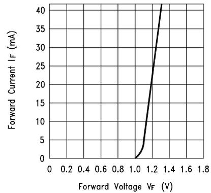
Fig.3 Collector Current vs. Forward Voltage
