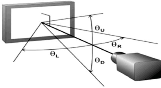
Note (6) Definition of Viewing Angle : Viewing angle range ( $C/R \geq 10$ )
