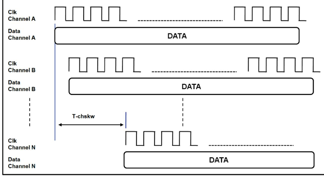
Note : DE should be synchronized with DE per each LVDS Channel and T-chskw < 16\* LVDS Clock Period
