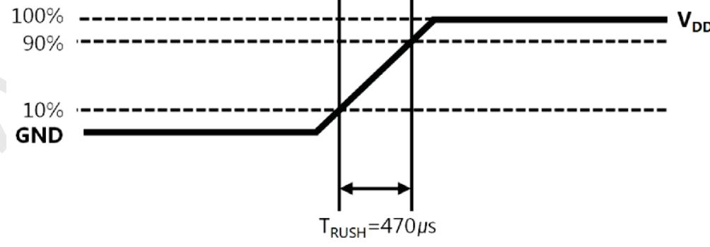
The rush current,  $I_{RUSH}$  can be measured when  $T_{RUSH}$  is  $470\mu\text{s}$ .
