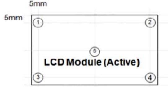
△T should be less than 10°C ( $\Delta T = |T_{CENTER} - T_{CORNER}|$ )
