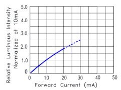
Fig.4 Relative Luminous Intensity vs. Forward Current
