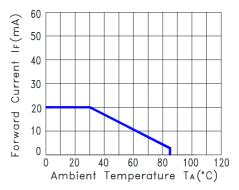
Fig.2 Forward Current Derating Curve
