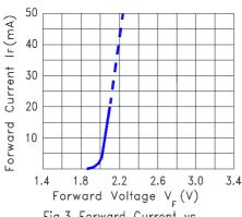
Fig.3 Forward Current vs. Forward Voltage
