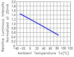
Fig.5 Relative Luminous Intensity vs. Ambient Temperature
