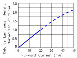
Fig.4 Relative Luminous Intensity vs. Forward Current
