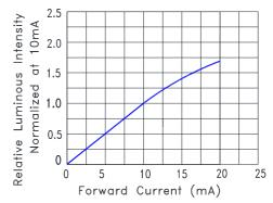
Fig.4 Relative Luminous Intensity vs. Forward Current
