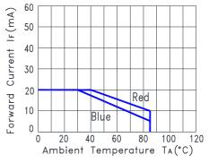
Fig.2 Forward Current Derating Curve
