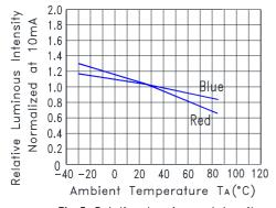
Fig.5 Relative Luminous Intensity VS. Ambient Temperature
