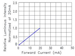
Fig.4 Relative Luminous Intensity vs. Forward Current
