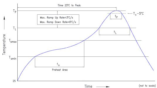
Note: Excessive soldering temperature and/or time might result in deformation of the LED lens or catastrophic failure of the LED.
