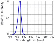
Fig.1 Relative Intensity VS. Wavelength
