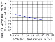
Fig.5 Relative Luminous Intensity VS. Ambient Temperature
