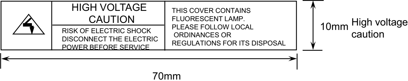
High voltage caution label
