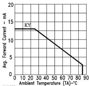
Fig5. MAX. AVERAGE FORWARD CURRENT VS. AMBIENT TEMPERATURE.
