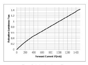
Fig 4. Relative Luminous Flux
