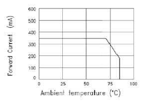
Fig 6. Forward Current Derating Curve
