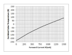
Fig 5. Correlated Color Temperature (CCT)Shift
