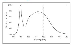
Fig 1. Relative Spectrum of Emission
