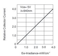
FIG.4 RELATIVE COLLECTOR CURRENT **VS IRRADIANCE**
