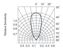
FIG.5 RELATIVE RADIANT SENSITIVITY vs. ANGULAR DISPLACEMENT
