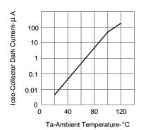
FIG.1 COLLECTOR DARK CURRENT **VS AMBIENT TEMPERATURE**
