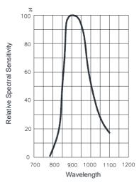
FIG.6 RELATIVE SPECTRAL SENSITIVITY **VS WAVELENGTH**
