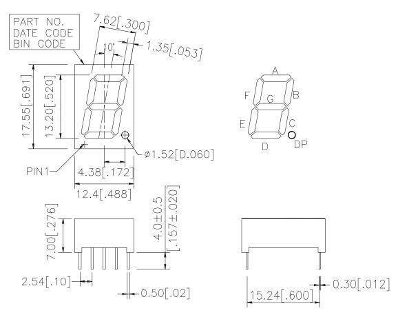
NOTES:1. All dimensions are in millimeters. Tolerances are  $\pm$  0.25 mm (0.01") unless otherwise noted. 2. Pin tip's shift tolerance is  $\pm$  0.4 mm.
