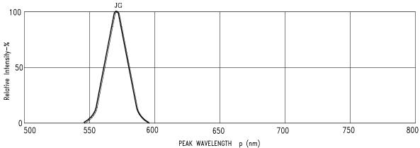
PEAK WAVELENGTH p (nm) Fig1.Spectral Emission
